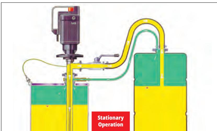
Concern about air pollution has never been so widespread as it is today. Acting on its sense of environmental responsibility, Lutz has further developed its emission proof drum adapter as a complete gas displacement system. Harmful gases and vapours created when transporting hazardous media remain practically in a closed system while themselves ensuring the necessary pressure compensation.
