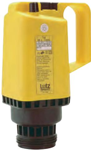
Double insulation in keeping with type of protection class II, splash water protected in keeping with IP 24, double-pole ON/OFF switch and single-pole thermal overcurrent release. 5 m connection cable with plug. Not explosion proof.
