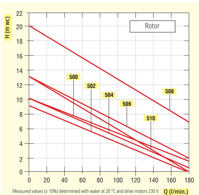
Please remember that the flow rate is reduced as the **viscosity** increases. The **density** of the pumped liquid similarly affects the flow rate, though to a lesser extent.
