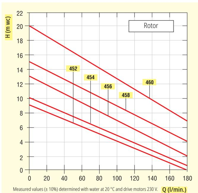
Please remember that the flow rate is reduced as the **viscosity** increases. The **density** of the pumped liquid similarly affects the flow rate, though to a lesser extent.
